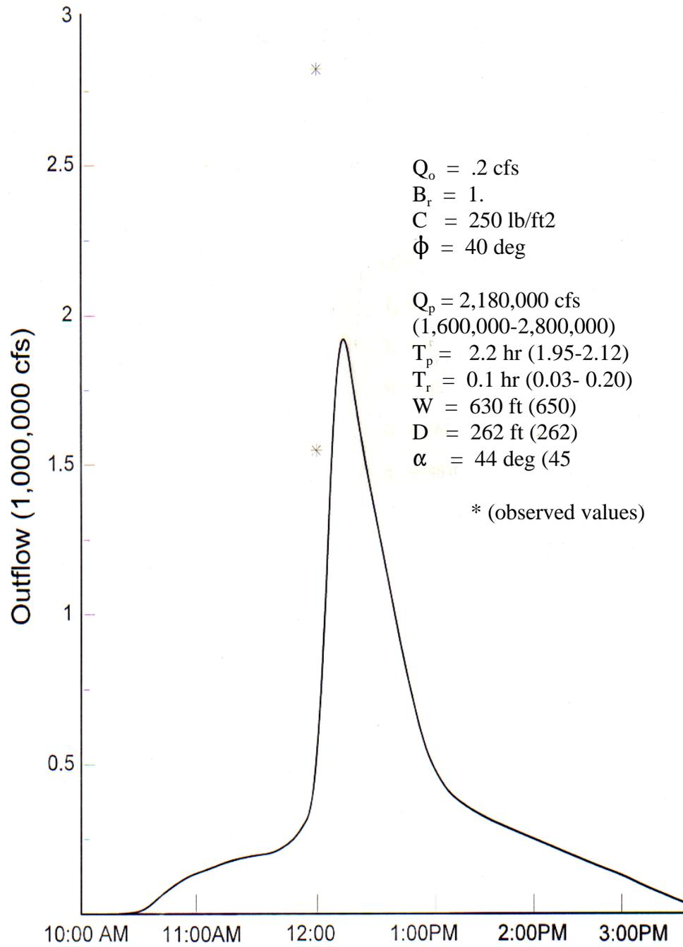
Teton Dam: Predicted and Observed Breach Outflow Hydrograph and Breach Properties
