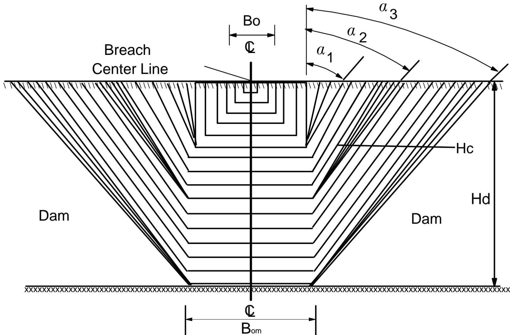
Figure 3. Front View of Dam with Breach Formation Sequence
