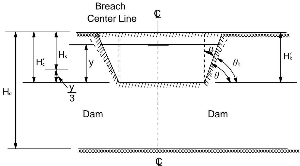
Figure 4. Front View of Dam with Breach
