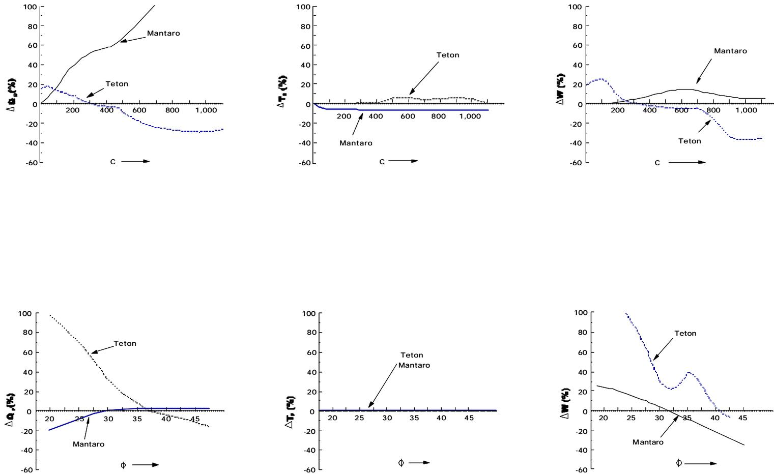
Figure 7. Sensitivity of Mantaro and Teton Predictions of Peak Outflow ( $Q_p$ ), Time to Peak ( $T_p$ ), and Breach Width ( $W$ ) to Changes in the Material Properties of the Dam: Cohesion ( $C$ ) and Internal Friction Angle ( $\phi$ )
