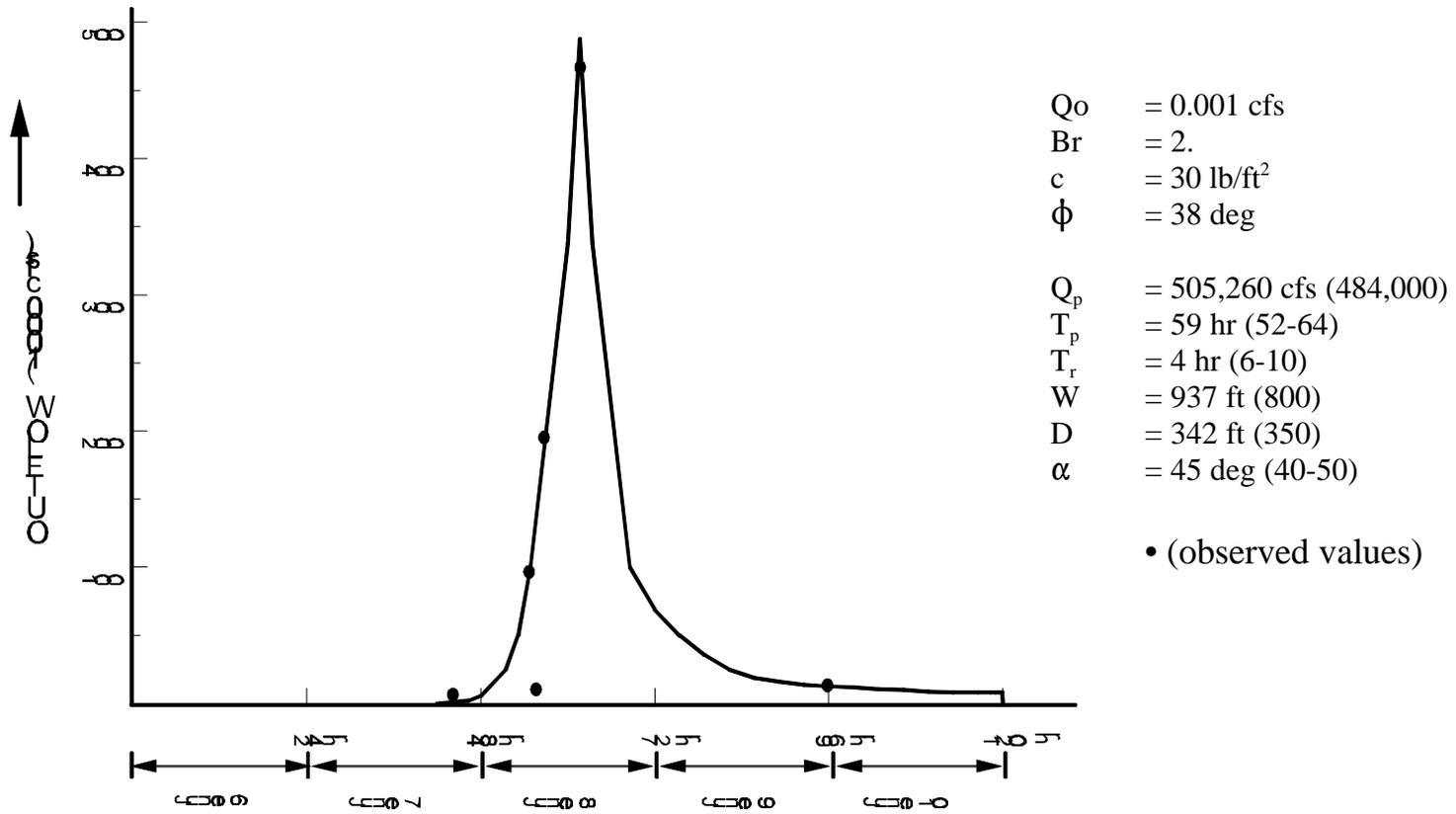
Figure 8. Mantaro Landslide Dam: Predicted and Observed Breach Outflow Hydrograph and Breach Properties
